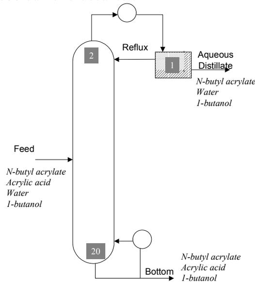
**Figure 2: Colonne of butyl acrylate purification**
