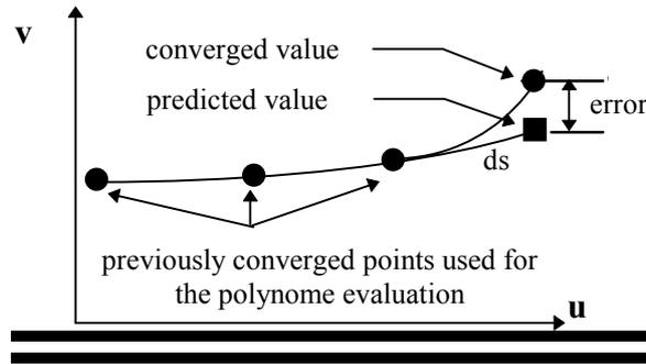
**Figure 1: Parameter operation path and curvilinear coordinate.**
