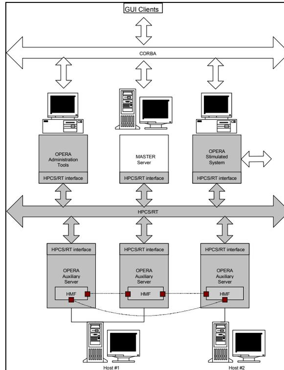
**Figure 1 - OPERA simulator physical deployment**
