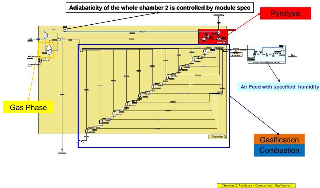
Figure 3: ProSimPlus<sup>®</sup> simulation diagram of the gasifier chamber 2
