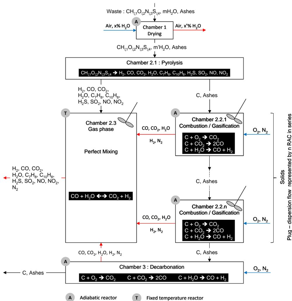
Figure 2: Schematic representation of the gasifier model
