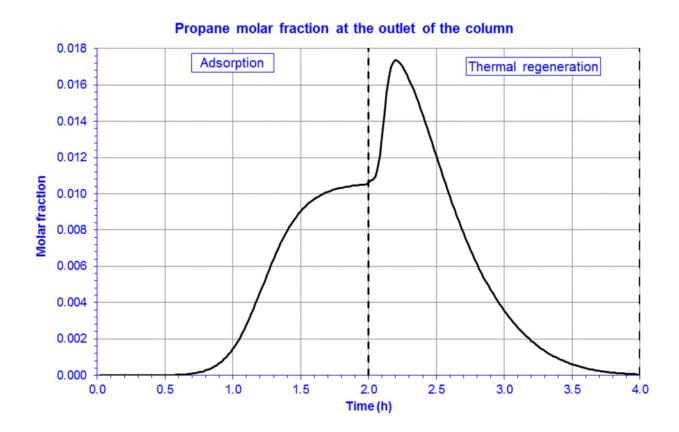
The above profile and other ones (temperature, pressure, flow rate, enthalpy, and compositions) are available for the column outlet stream at the end of the simulation from the outlet stream edition window ("Tabulated results..." button in the "Parameters" tab).
