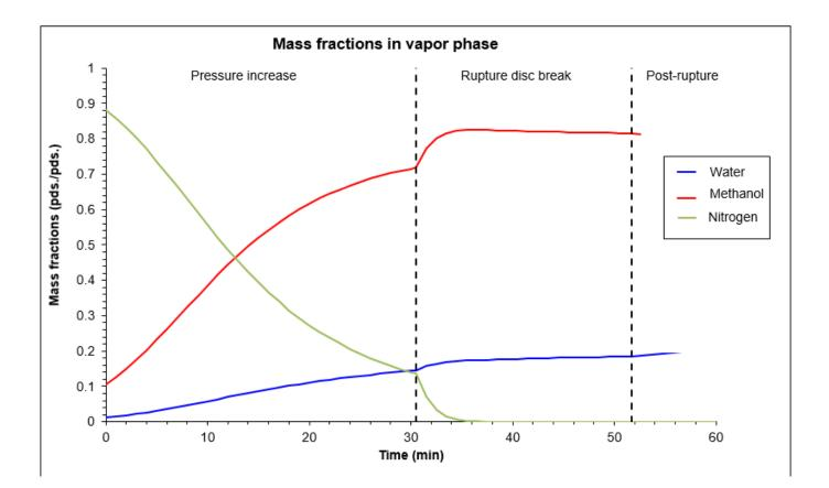
The following graph shows the evolution of the load in the reactor. It shows that almost 40% of the initial mass load is vented away when the rupture disc breaks out.
