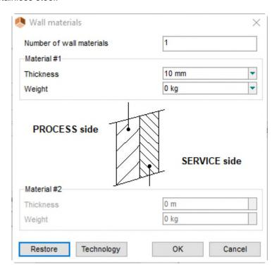
The thermal conductivity of stainless steel is considered to be equal to 19 W/m<sup>-1</sup>.K<sup>-1</sup>. The thermal conductivity is specified for each operating step.
