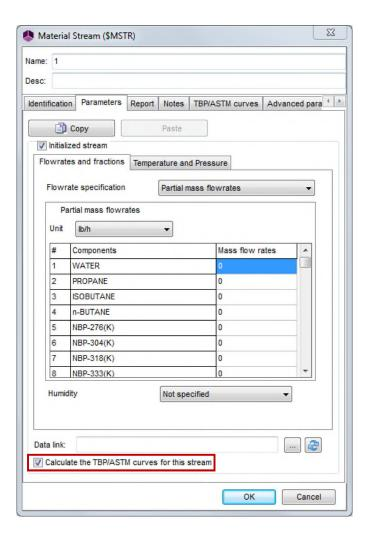
To reach this option the "Initialized stream" box has to be ticked and then unticked once the "Calculate the TBP/ASTM curves for this stream" box has been ticked.
