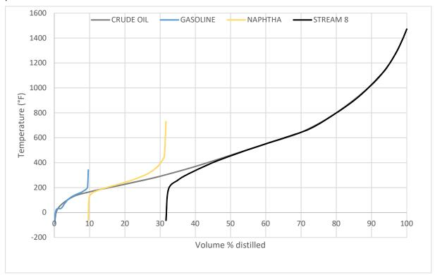
The following figure shows on a same graph the TBP at 760 mmHg curve of the stream 8 entering the main column C3 and the ones of the cuts obtained at the outlet of this column:
