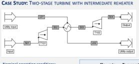
The intermediate heat exchanger increases the stream process temperature up to 770 K.
