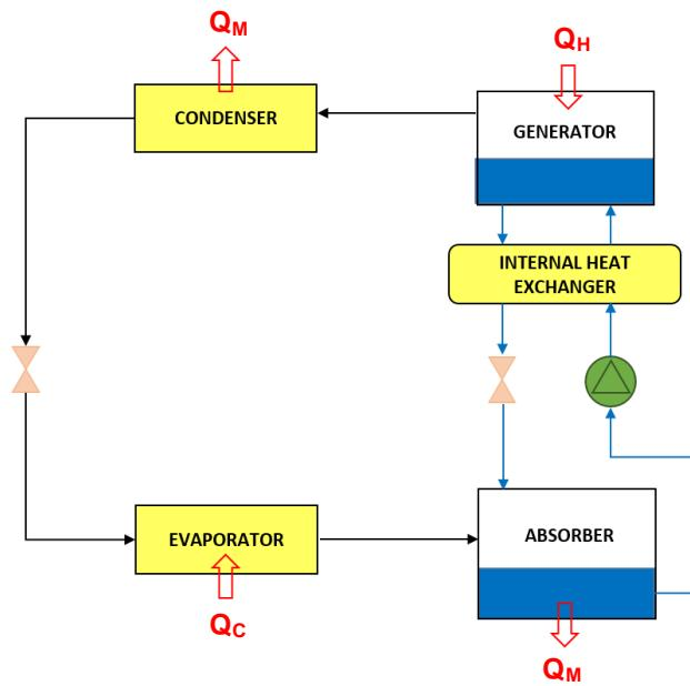
*Schematic of an absorption refrigerator*
