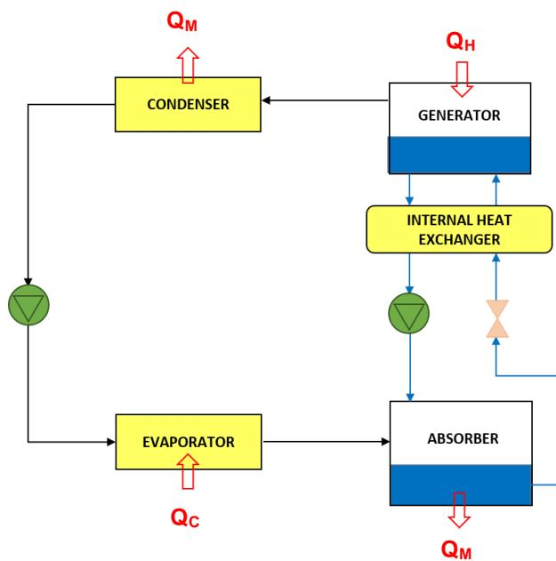
Schematic of an absorption heat transformer
