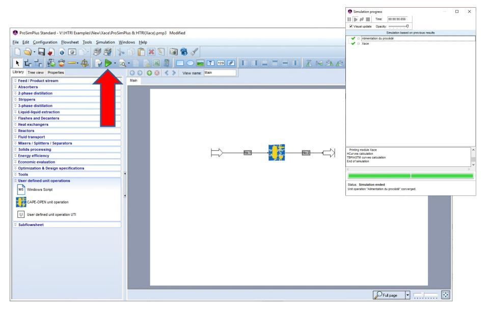
When the simulation is complete, you can edit the reports of the Xace heat-exchanger with a double-click on the corresponding icon:
